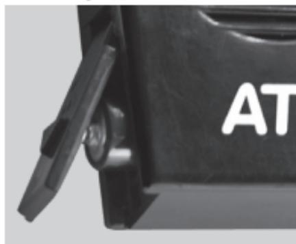
of the device. Slide the door down, until it clicks, to open the battery compartment. The negative ends of the batteries go in the compartment first.
