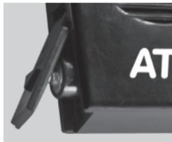
battery door is on the end of the device. Slide the door down, until it clicks, to open the battery compartment. The negative ends of the batteries go in the compartment first.
