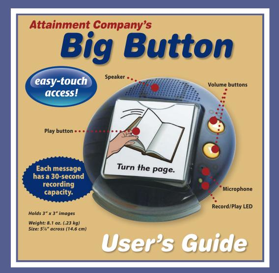
The **Big Button** is a powerful communication tool with a single large Play button. A removable transparent cap snaps onto the Play button and has an opening on top for sliding in overlays or icons. Remove the cap by firmly pulling up on the lip until it dislodges. Then pull on the top part of the cap to remove it. The cap extends nearly to the table surface, creating a large activation area with an extremely
